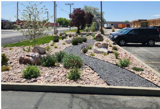
Example of permeable hardscaping and water-wise plantings in an industrial development.
