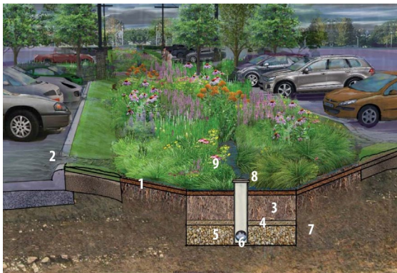
Cross-section diagram of bioretention design in a parking area.
